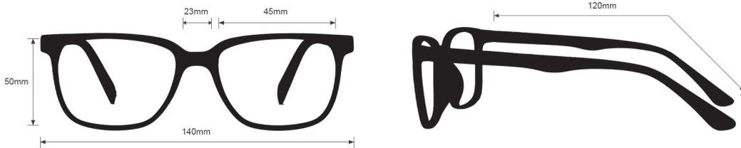
The Safety Glasses 21509 have a wrap-around frame made of high-quality plastic. The 21509 model is lightweight, highly durable, and impact resistant. Plus, it features rubberized nose pads and no-slips temples for superior comfort. These Safety Glasses are available in a black frame with two lens variations: clear or smoke. They also meet rigorous ANSI Z87+ and EN 166 industry standards, offering high impact certification for optimal protection.
