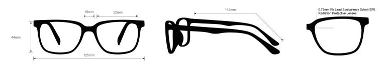
The Ray Ban radiation glasses Elliot feature high-quality, distortion-free SF-6 Schott glass radiation-reducing lenses with 0.75mm Pb lead equivalency protection. These Ray Ban lead glasses have clear CE Certified Lens and weigh 92g. Plus, the Elliot radiation glasses are prescription available. Made of high-quality plastic, they have a durable and lightweight square frame. These lead glasses feature a high bridge fit and are available in two color variations: polished havana and polished black.
