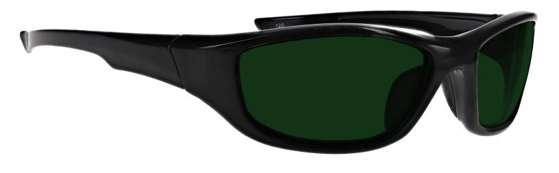
The Green Welding glasses 703 have a polycarbonate green welding filter shade 2.0, 3.0, 4.0, 5.0, 6.0, 8.0, that provides torching and brazing protection. These green torching glasses are ANSI Z87.1, EN 166 and EN 169 approved, and have CE certified lens
