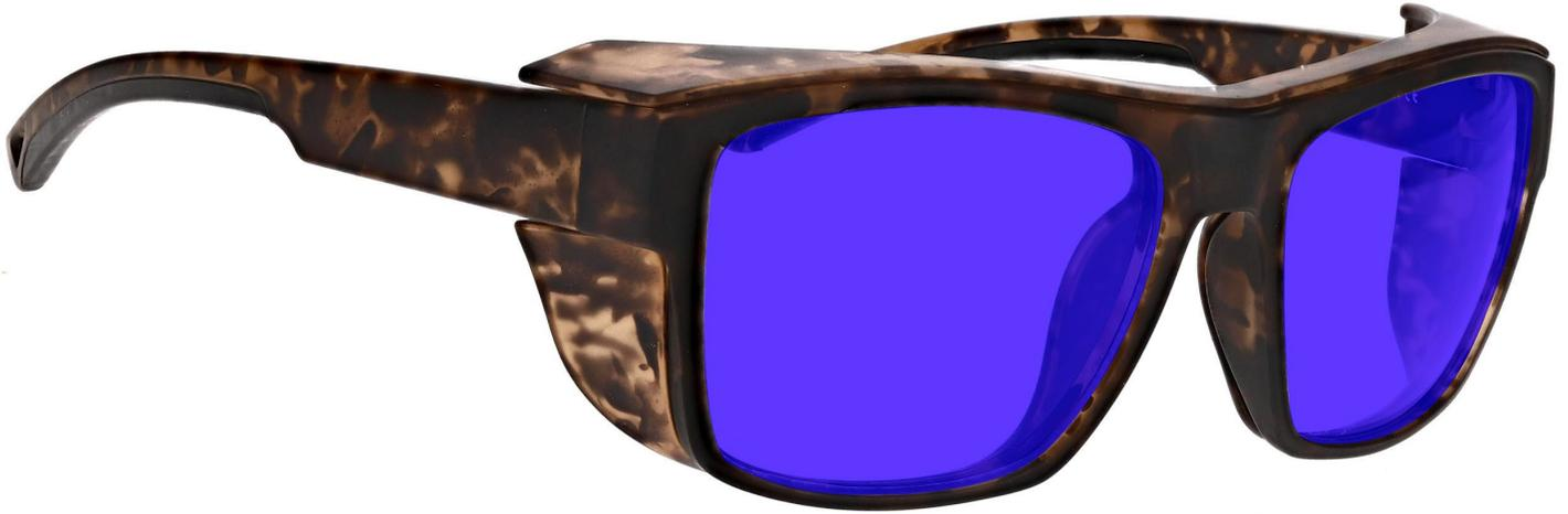
The lampworking glasses Sodium Flare Poly have a polycarbonate purple glassworking lens that provides good color recognition for soft glass. These frameworking glasses offer excellent UV blocker, excellent sodium flare blocker, and good clarity. Recommended for those who work with lampwork or hot glass in small pieces.
