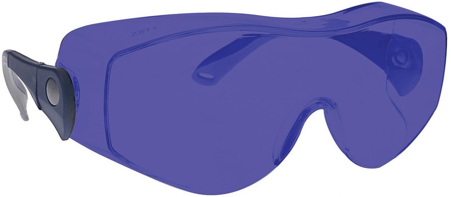
The lampworking glasses Sodium Flare Poly have a polycarbonate purple glassworking lens that provides good color recognition for soft glass. These frameworking glasses offer excellent UV blocker, excellent sodium flare blocker, and good clarity. Recommended for those who work with lampwork or hot glass in small pieces.
