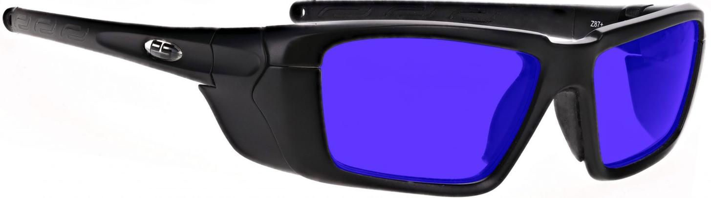
The lampworking glasses Sodium Flare Poly have a polycarbonate purple glassworking lens that provides good color recognition for soft glass. These frameworking glasses offer excellent UV blocker, excellent sodium flare blocker, and good clarity. Recommended for those who work with lampwork or hot glass in small pieces.
