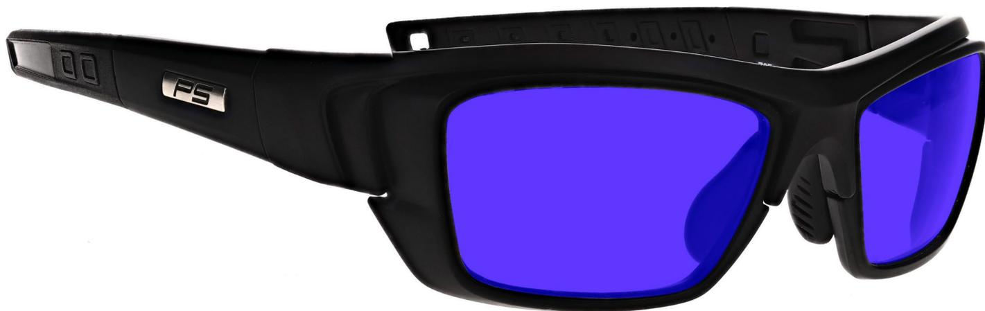
The lampworking glasses Sodium Flare Poly have a polycarbonate purple glassworking lens that provides good color recognition for soft glass. These frameworking glasses offer excellent UV blocker, excellent sodium flare blocker, and good clarity. Recommended for those who work with lampwork or hot glass in small pieces.
