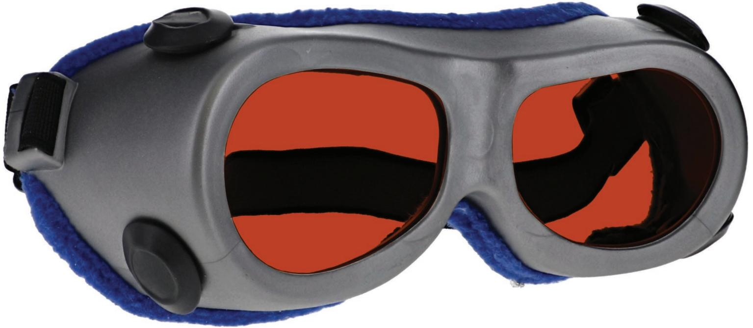
The YAGA laser safety glasses have a polycarbonate dark orange lens filter that provides laser protection. These laser glasses have visible light transmission of 12%. In addition, the YAGA laser safety glasses have ANSI Z87.1 and ANSI Z136.1 safety standards. These laser safety goggles 55 is a durable and lightweight fitover goggles frame. Made of high-quality plastic, the 55 laser safety goggles feature strap. These Phillips Safety laser safety goggles are available in silver.
