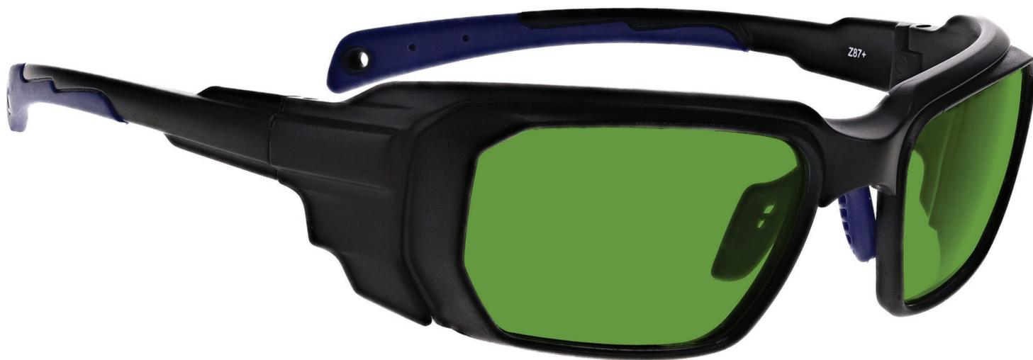
The D1500 laser safety glasses have a polycarbonate green lens filter that provides laser protection. These laser glasses have visible light transmission of 16%. In addition, the D1500 laser safety glasses have ANSI Z87+ and ANSI Z136.1 safety standards. These laser safety glasses 16001 is a durable and lightweight wrap around frame. Made of high-quality plastic, the 16001 laser safety glasses feature adjustable nosepads. These Phillips Safety laser safety glasses are available in black/blue.
