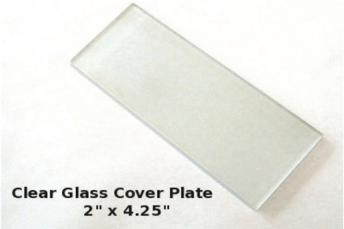
The Clear Glass Cover Lens | Small 2 x 4.25 is a replacement cover lens for welding helmets made of non-hardened clear glass. The high-quality material of this Phillips Safety lens offers superior protection from dust, weld spatter and impact. These Clear Glass Cover lenses have a small rectangular shape with dimensions of 2" H x 4.25" W and 2 mm of thickness. In addition, they fit most brand name helmets.
