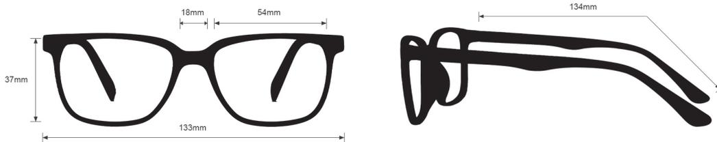
The Safety Glasses OP30 are a rectangular frame made of high-quality plastic. The OP30 model is lightweight, highly durable, and impact resistant. Plus, it features removable side shields. These Safety Glasses are available in black and tortoise. They also meet rigorous industry standards, with ANSI Z87+ and EN 166, offering high impact certification for optimal protection.
