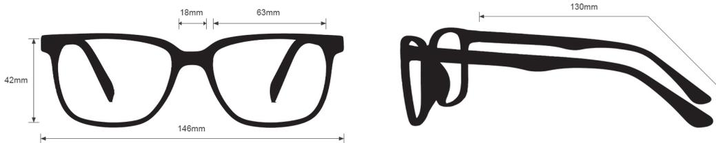
The Safety Glasses 17001 are a rectangular, wrap around frame made of high-quality plastic. The 17001 model is lightweight, highly durable, and impact resistant. Plus, it features rubberized temples. These Safety Glasses are available in black/green. They also meet rigorous industry standards, with ANSI Z87+ and EN 166, offering high impact certification for optimal protection.
