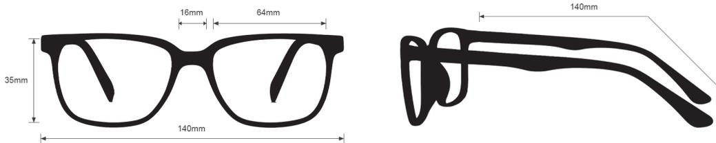
The Safety Glasses 1205 are a wrap around frame made of high-quality plastic. The 1205 model is lightweight, highly durable, and impact resistant. Plus, it features rubberized nose pads and rubberized temple bars. These Safety Glasses are available in blue and black. They also meet rigorous industry standards, with ANSI Z87.1 and EN 166, offering high impact certification for optimal protection.
