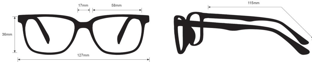
The Safety Glasses 116 are a rectangular, wrap around frame made of high-quality metal. The 116 model is lightweight, highly durable, and impact resistant. Plus, it features adjustable silicone nosepads, rubberized temples, and spring hinges. These Safety Glasses are available in black and silver. They also meet rigorous industry standards, with ANSI Z87.1 and EN 166, offering high impact certification for optimal protection.
