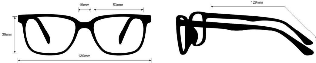
The Safety Glasses T9603 are a rectangular frame made of high-quality plastic. The T9603 model is lightweight, highly durable, and impact resistant. Plus, it features silicone nose pads, rubberized temples, removable silicone gasket, and integrated side shields. These Safety Glasses are available in black with clear, and orange with clear. They also meet rigorous industry standards, with ANSI Z87+, CSA Z94.3 and EN 166, offering high impact certification for optimal protection.
