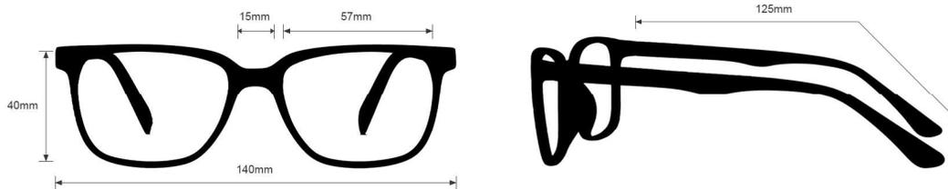
The Safety Glasses 15011 are a square frame made of high-quality plastic. The 15011 model is lightweight, highly durable, and impact resistant. Plus, it features rubberized nose pads, rubberized temple bars, adjustable nose pads and permanent side shields. These Safety Glasses are available in eight color variations. They also meet rigorous industry standards, with ANSI Z87+, CSA Z94.3 and EN 166 certified, offering high impact certification for optimal protection.
