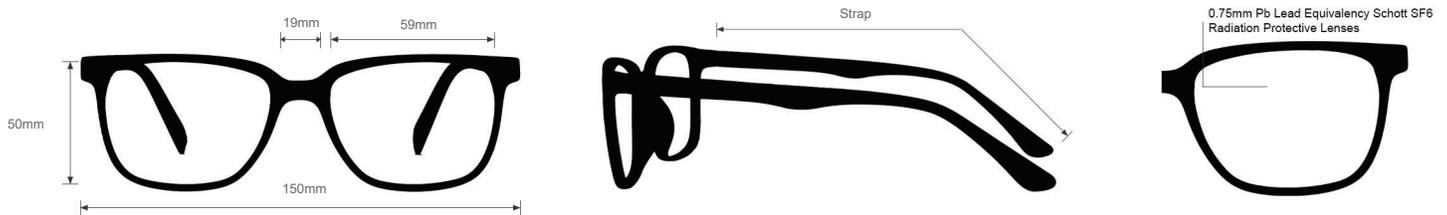
The radiation glasses 55 feature high quality, distortion-free SF-6 Schott glass radiation-reducing lenses with 0.75mm Pb lead equivalency protection. The 55 lead glasses have clear CE Certified Lens and weight 158 g. These radiation goggles 55 are non-prescription. Made of high-quality plastic, it is a durable and lightweight fitover goggles frame. The 55 radiation goggles feature strap. These Phillips Safety radiation goggles are available in silver.
