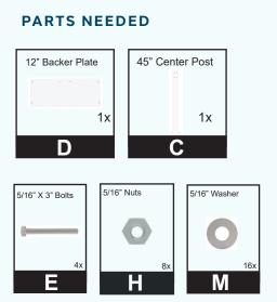
7. Attach washers M and nuts H to the front side and tighten.
